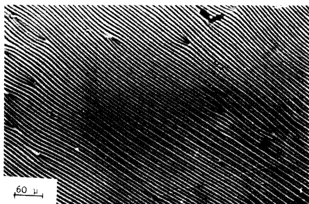
Figure 4. Micrographs of a pure fractionated anisotropic phase: (a) thickness of the layer about 50 \mu\text{m} ; (b) same sample at a lower thickness.
